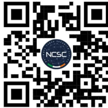
A QR code is a type of barcode that stores information, such as website links. QR codes are very easy to create and can be scanned using the camera on a smartphone to access the information stored in the QR code.
